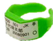
Radiophoto-luminescence (RPL) glass dosimeter (badge type)
